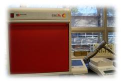
test sample is placed in a crucible which is weighed pre and post ashing and recorded in the controller. We have the ability to use our Massspectrometer to analyze the vapor from the ashing process.
