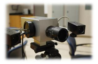
Shearography - NDT Measurement Systems | Shearography - NDT Systems for Flaw Detection in Composite Materials - Dantec Dynamics Typical flaws detectable in Composite Materials with Shearography are:
