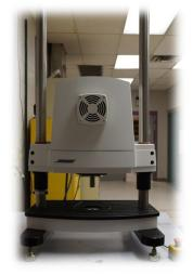
ElectroForce<sup>®</sup> multi-specimen fatigue test systems are designed to provide tension-tension, or compressioncompression displacement controlled loading for small soft structures and devices, such as stents, stent structures, stented grafts, vena cava filters, septal patch structures or other similar devices.
