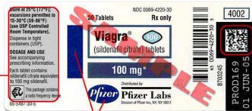
EPCglobal Logo and RFID Tag location (tag is under label)
