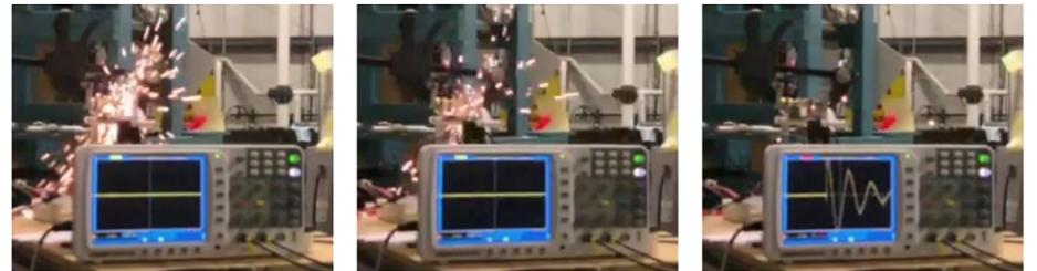
**Figure 5.** Sequence of screenshots from a video of the Can Crusher experiment and  $\dot{B}$  probe trace on an oscilloscope.
