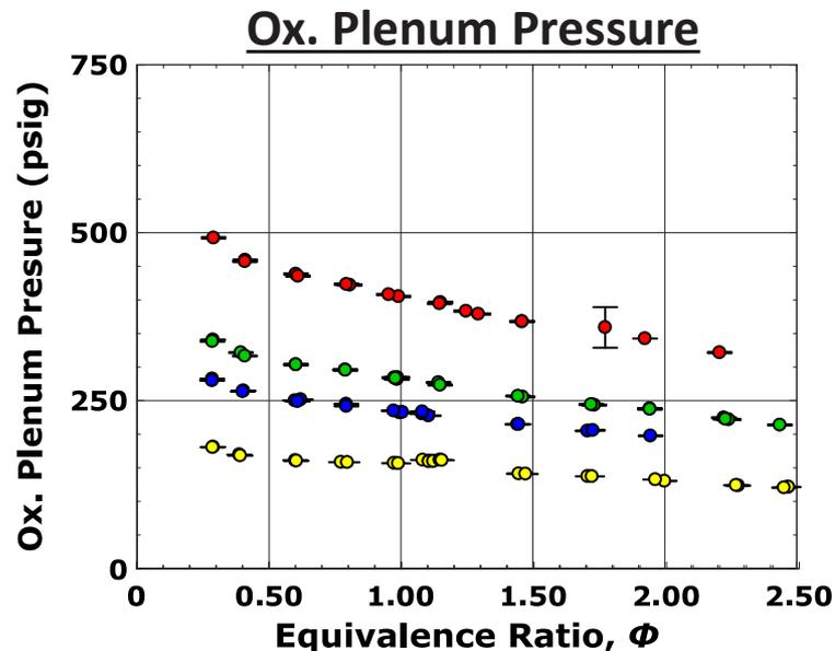
2.5A corresponds to a fuel pressure drop that is ~5X smaller than for 1.0A, while the ox. pressure drop is 3X smaller.
