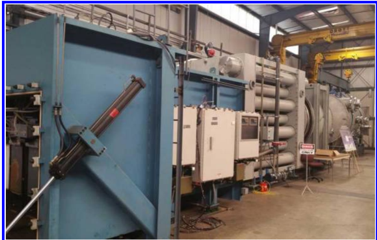
Figure 26. The 3 Terrawatt, DECADE Module 2 Pulse Power Machine
