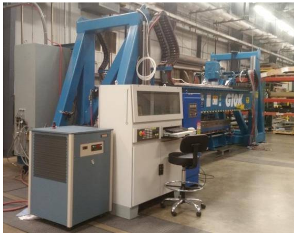
Figure 24. NovaTech G10K/ Large Panel Gantry FSW/TSW equipped with high torque motor and auxiliary induction heating
