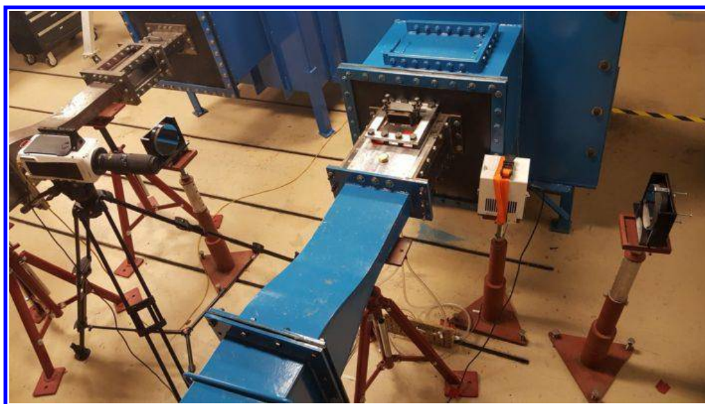
Figure 10. Supersonic Wind Tunnel research test section, teaching demonstration test section, Schlieren and shadowgraph visualization apparatus, and associated components.
