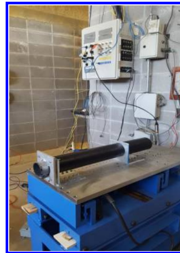
Figure 9. New UAH Rocket Test Stand (With Solid Rocket Motor) 13
