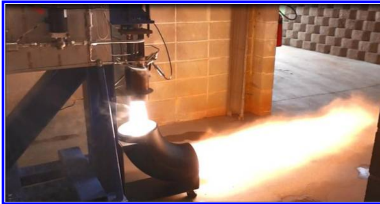
Figure 8. New UAH Vertical Rocket Test Stand (With LOX Liquid Rocket Engine)
