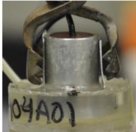
Solid Propellant Sample
