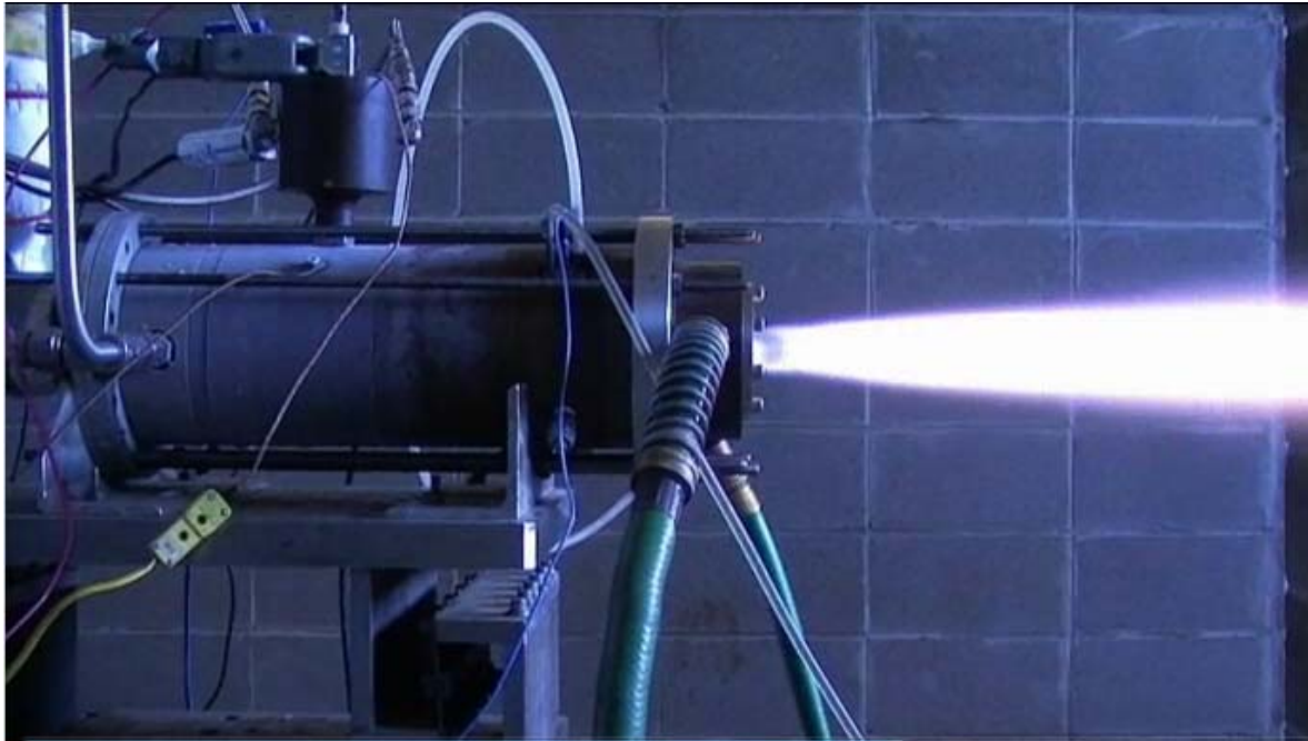
Figure 13. Cryogenic Oxygen Gaseous Methane Rocket Engine Firing at the UAH Propulsion Test Facility
