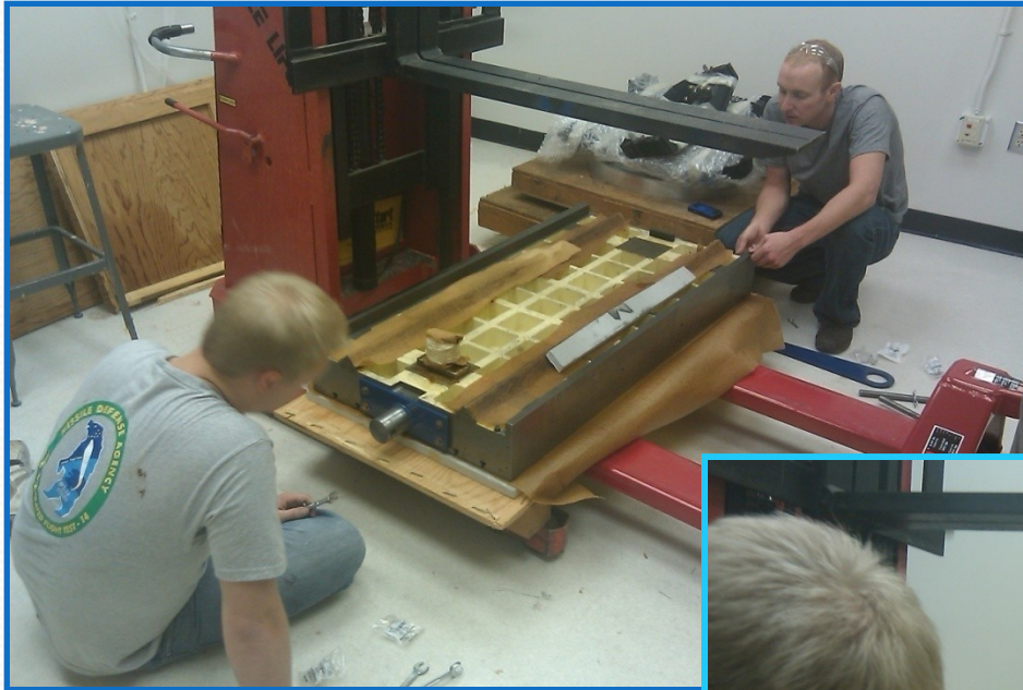
Bolting Bearings to Slide
