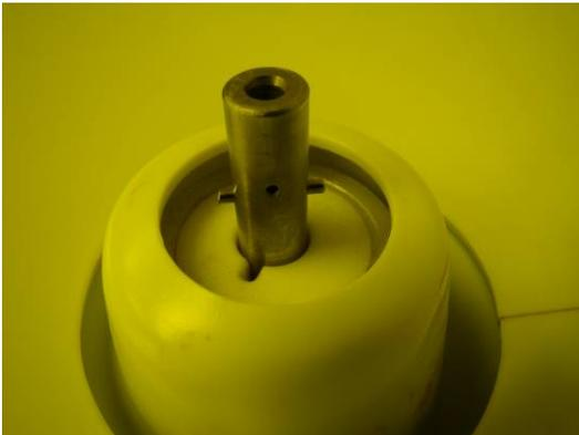
about 500 RPM by adjusting the dial below the illuminated SPREAD button so that it displays about 50. If the SPREAD button is not lit press it once which enable a spread cycle and set the timer for about 20 seconds, just enough time to see observe the sample as it spins.
