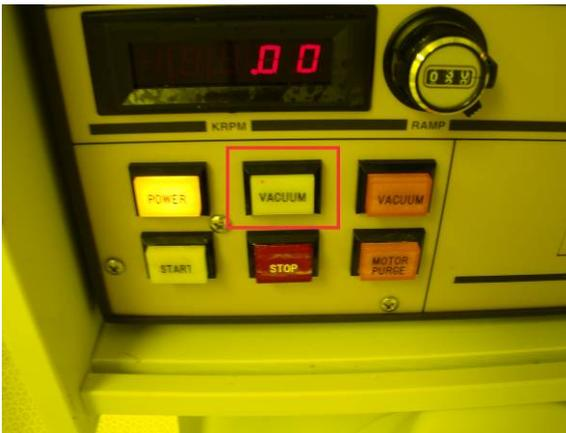
Press VACUUM to release vacuum, adjust your sample as necessary, press VACUUM again to reactivate it and try it again.
