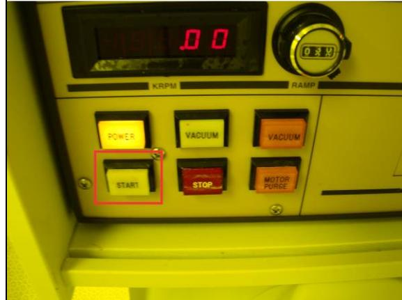
When the spin is complete remove the cover, press VACUUM, remove your sample, clean out the bowl, recover the spinner and press POWER to turn the machine off.
