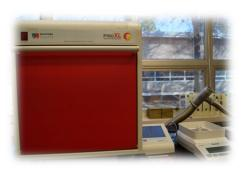
test sample is placed in a crucible which is weighed pre and post Ashing and recorded in the controller. We have the ability to use our Massspectrometer to analyze the vapor from the Ashing process.
