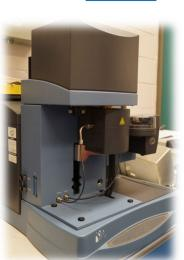
In thermogravimetry weight changes of a substance which occur during a controlled temperature program and in a defined gas atmosphere are measured. In the Difference Thermal Analysis (DTA), temperature changes of a substance
