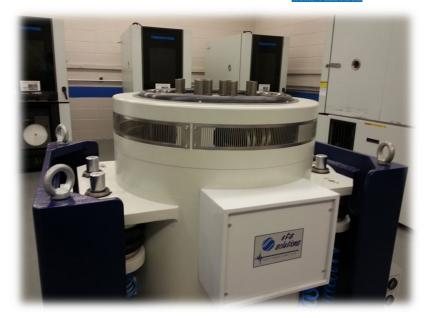
The dynamic vibration system is designed to simulate vibration or shock that an item will be subjected when in its normal application. The system can perform random vibration, sine vibration, sine on random vibration, sine on sine vibration, and all varieties of mechanical shock. The controller has the capability to interface with the output of a recording device permitting testing under the actual vibration profile of the target component under use.
