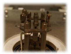
dependent behavior. The DMTA is a mechanical spectrometer that measures the stress/strain relationship of the material being tested. The DMTA can be used to test curing cycles and efficiency for thermosets and elastomers. It can be used for quality control of plastics and
