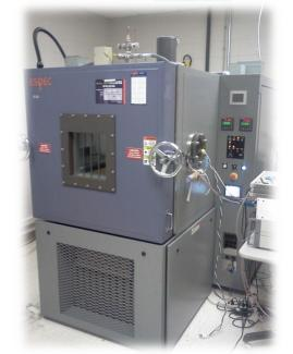
altitudes as well as being able to control the temperature. The chamber also has a humidity mode of operation where you can subject the samples to different humidity and temperature ranges. While in altitude mode if you have sensitive electronic equipment, the chamber can keep greater than 20% RH while testing at or below 5,000 feet. This will allow you to safely turn on sensitive electronics and not cause static arcing or discharge.
