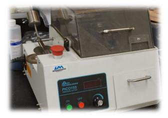
The PICO 155 is a precision wafering saw with touch controls. It has variable cutting speed from 50-1500 rpm with a digital
