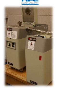
molded parts, coatings, paint, ink on substrates, thin films, and fiber testing. Current use is to test the properties of carbon fiber.
