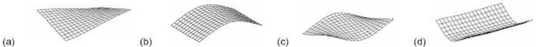
AR = 1.5. Finite element results for a 152.40 mm x 228.60 mm (6 in. x 9 in.) GRSPMC plate, (a) 1st mode, frequency = 269.50 Hz, (b) 2nd mode, frequency = 410.86 Hz, (c) 3rd mode, frequency = 674.20 Hz, (d) 4th mode, frequency = 913.14 Hz.
