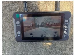
40CH FPV Transmitter and a <u>Sologood FPV Monitor</u> receiver to display the footage on a handheld device.
