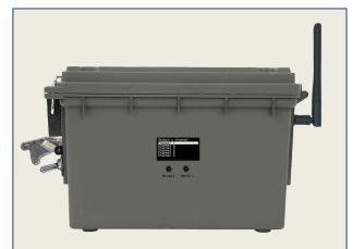
We chose a 1200mAh rechargeable battery to allow our system to work for around 6 hour before needed recharged. The Antenna was chose for the fact it is able to easily be attached to the Arduino, and is able to transmit the 2.4Ghz signal needed.
