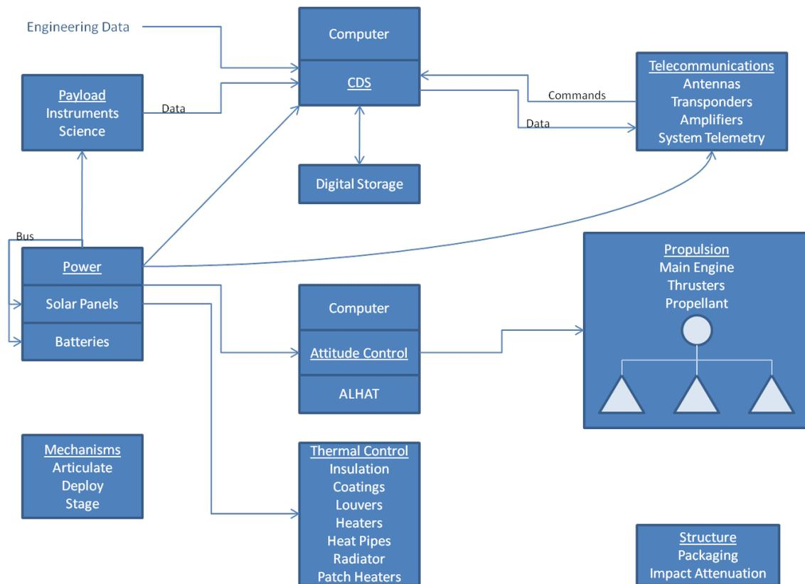
Figure 17 RAILL Block Diagram
