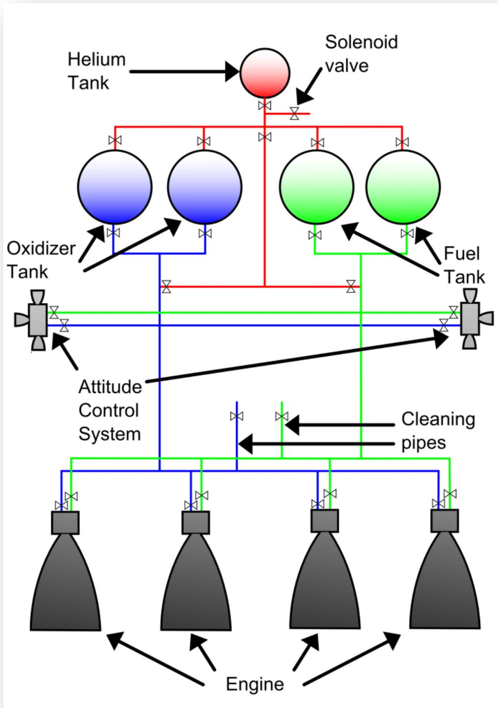
Figure 30: Simplified Hydraulic Diagram
