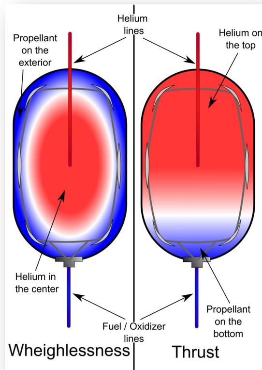
**Figure 31: The repartition of helium and propellant**
