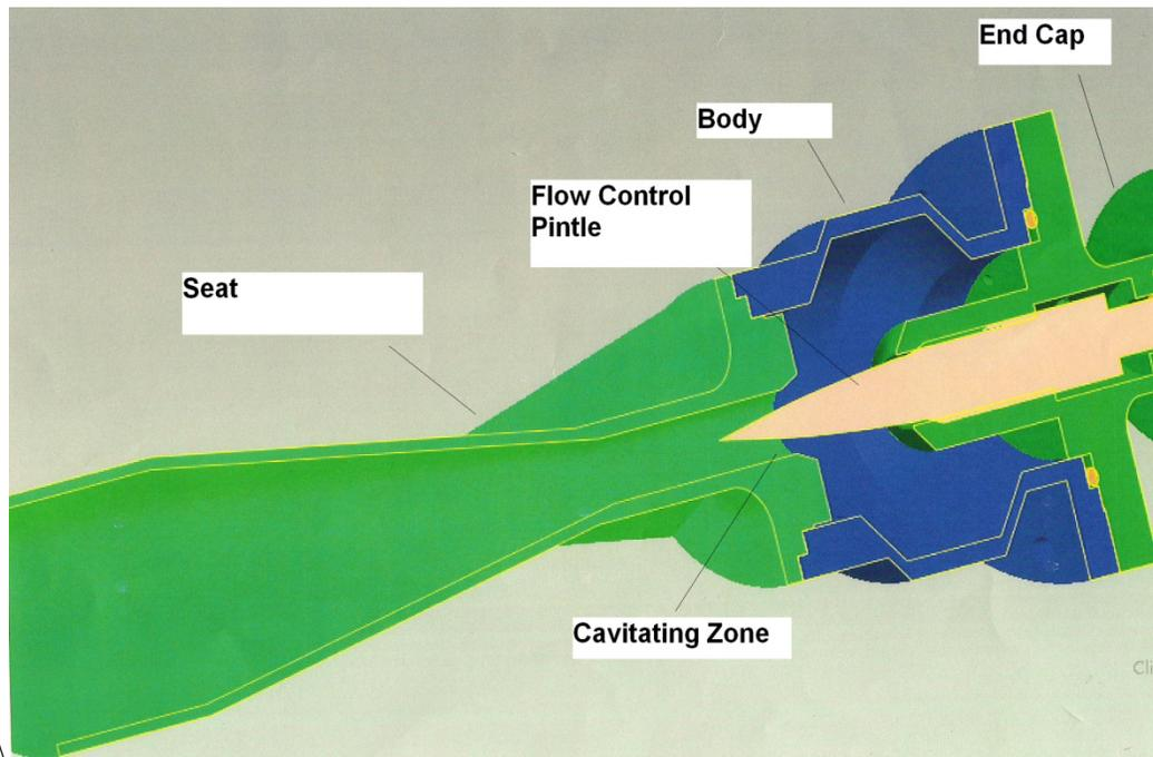
Figure 2. TCaV cross section.
