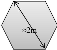
For a given cylindrical fairing it offers more room than a cubic one. It allows the big spherical fuel tanks to fit in without any waste of space.
