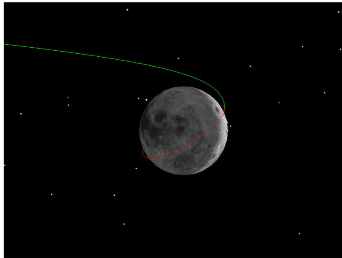
**Figure 13** Lunar Orbit Insertion Trajectory
