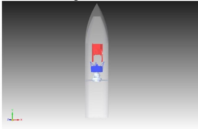
Figure 16 Spacecraft Stack in Shroud
