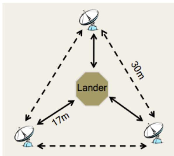
**Figure 15:** Arrangement of Science Packages
