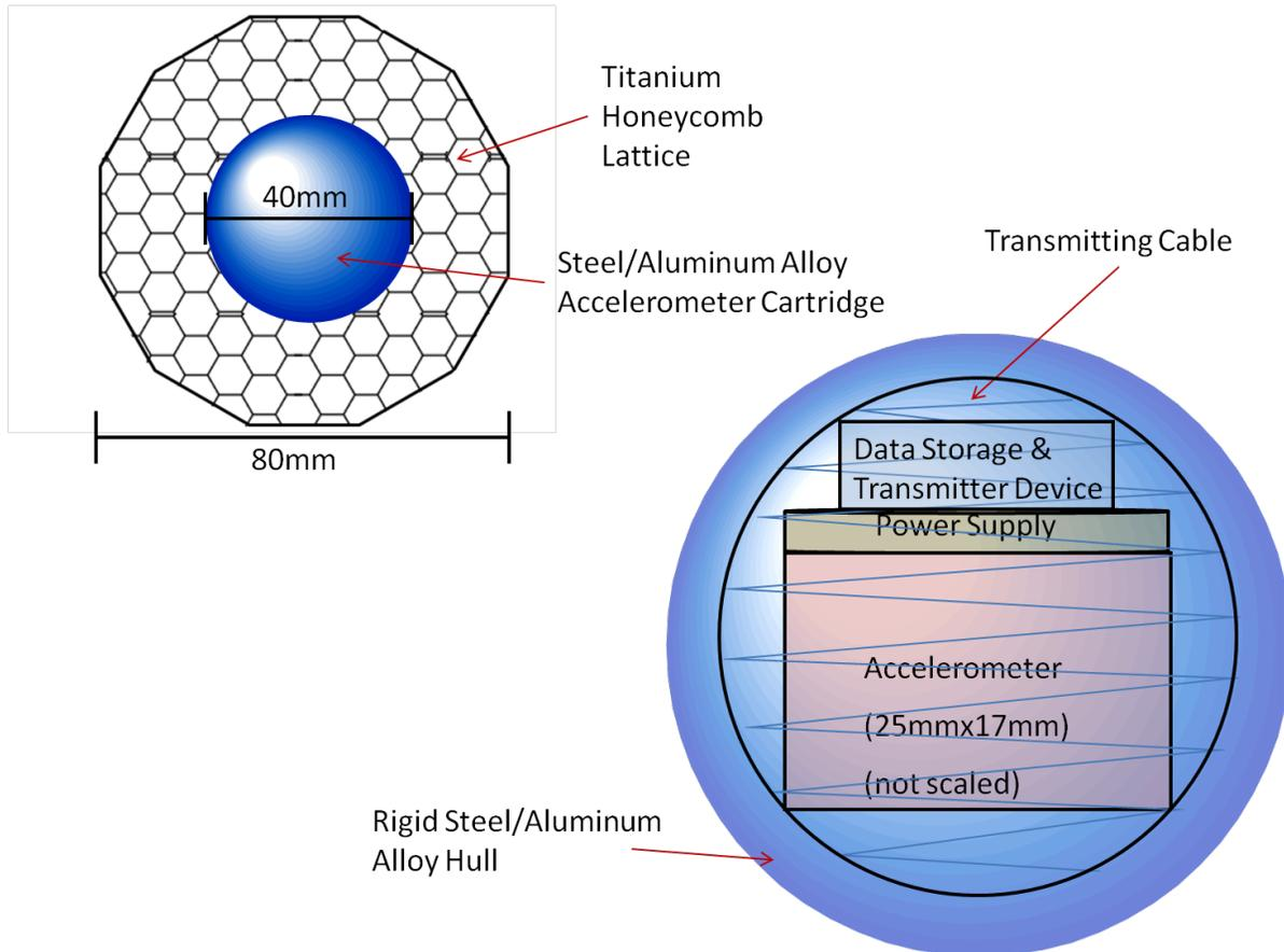
Figure 1. – Accelerometer Cartridge Layout
