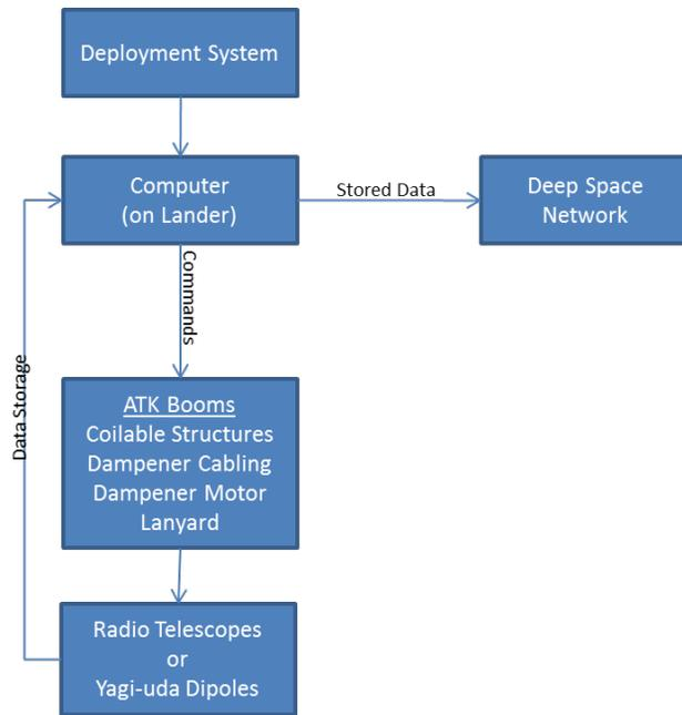
**Figure 20** Deployment System Block Diagram
