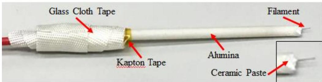
Figure 3.8 Example of a single Langmuir probe used in this study.
