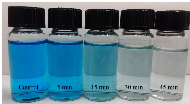
Figure 52. Samples treated at 8 kV, 10 kHz, 1 \mu s, and 2 slm for 0, 5, 15, 30, and 45 minutes showed the steady degradation of MB dye.
