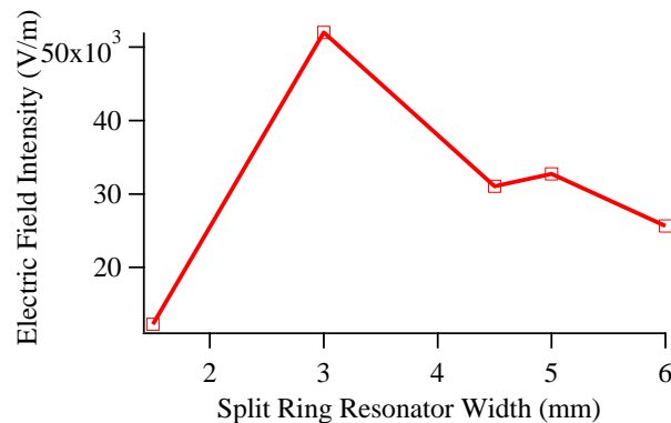
Figure 27. Simulation results of electric field intensity versus SRR width.
