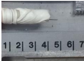
Figure 21. Langmuir probe from UAH PRC (millimeter units).
