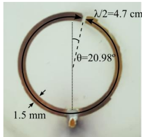
Figure 3. Example of split-ring resonator device used.
