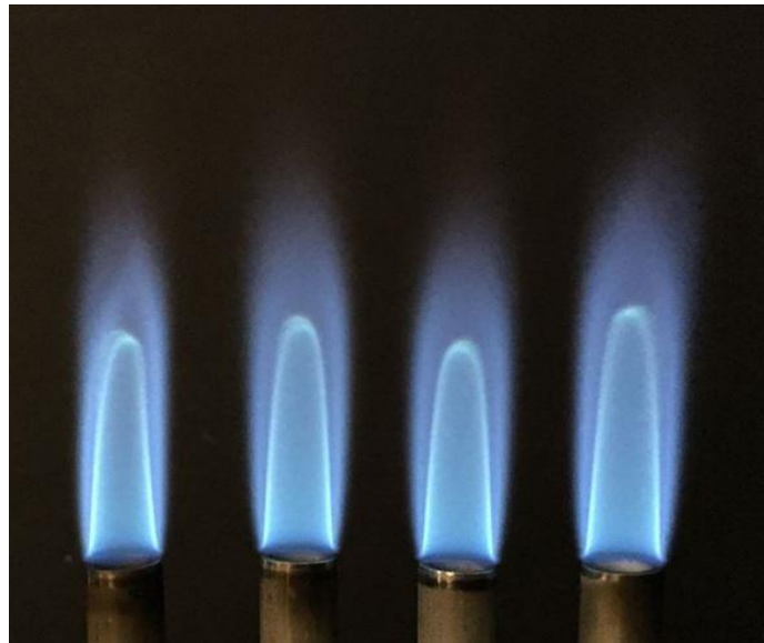
Figure 3.5 Example picture of the multi-element burner flames showing a uniform and evenly distributed flames with only small ambient perturbations.
