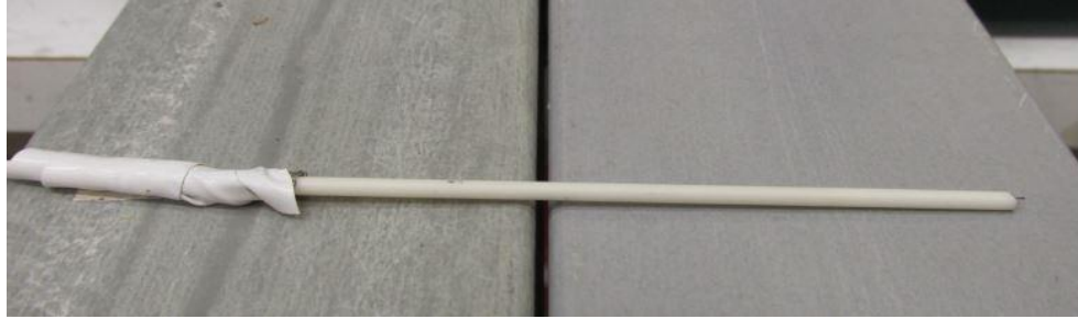
Figure 3.8 Example of a single Langmuir probe used in the present work.
