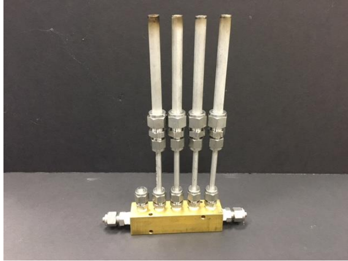
Figure 3.4 Multi-element burner setup using a brass manifold for investigating the effect of DC electric fields on the lean flammability limit and blowoff velocity of a flame.
