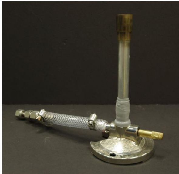
Figure 3.3 Bunsen-type burner used for observing the flame dynamic response and ion number density measurements.
