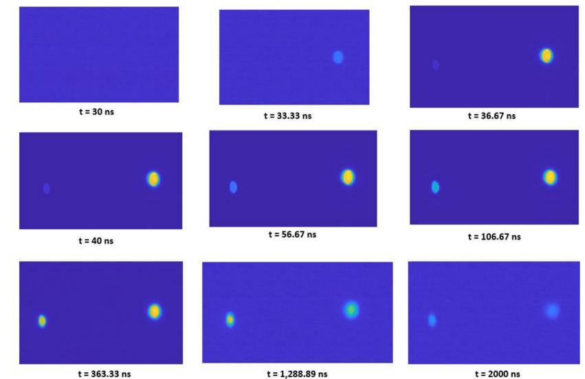
Figure 6. Time-Elapsed Plasma Expansion (760 Torr, 400 mJ).
