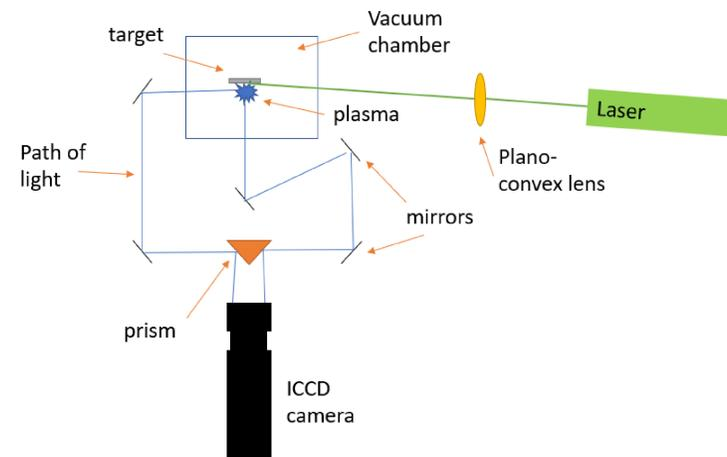
Figure 3. Schematic of Dual-View Plasma Imaging Setup.
