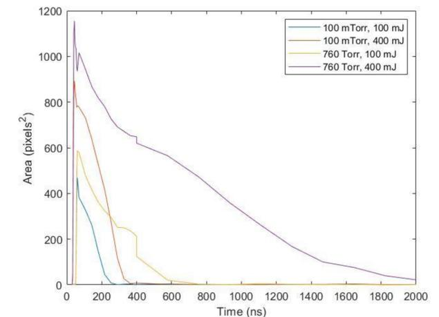
Figure 5. Area vs. Time for Front View Plasma Expansion.
