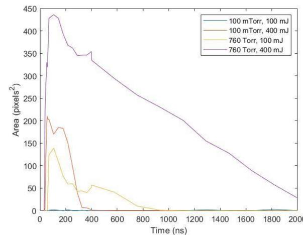
Figure 4. Area vs. Time for Side View Plasma Expansion.
