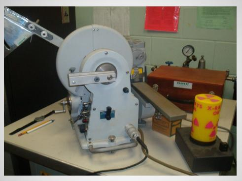
This is an OLD open beam X-ray diffraction device. New diffraction X-Ray devices for UAH research must be contained in a fully shielded interlocked cabinet.
