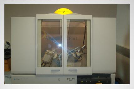
The x-ray tube, detector, sample are contained in a housing that provides shielding to the user and others in the lab. The access doors are interlocked and will shut off the x-rays when opened. The large viewing area is made possible by using leaded glass or Plexiglass
