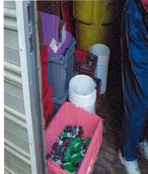
Picture 10 - Universal Waste Storage Shed#1 – Storage of open, unlabeled and not dated containers of spent alkaline, lithium and lead acid batteries
