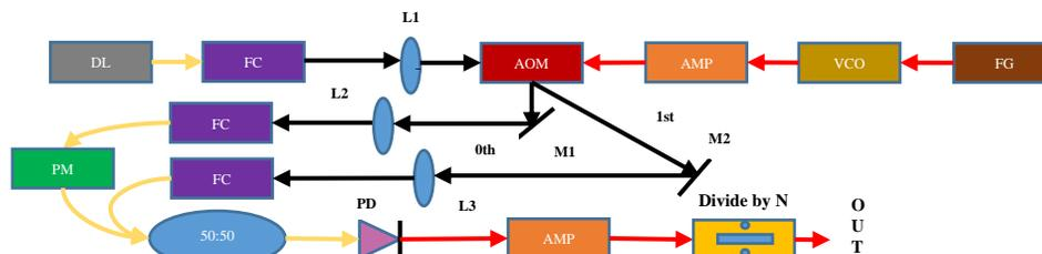
Fig. 1. Schematic of experimental setup. DL: Diode laser; FC: Fiber Collimator; M1,M2: Mirrors; L1,L2,L3: Collimating lenses; AOM: Acousto-optic modulator; Amp: Amplifier; VCO: Voltage-controlled oscillator; FG: Function generator; PM: Electro-optic phase modulator; 50:50: Fiber coupler; PD: Photodiode; Divide by N: EFD; Yellow arrow: single mode fiber; Black arrow: free space path; Red arrow: Electrical cable.
