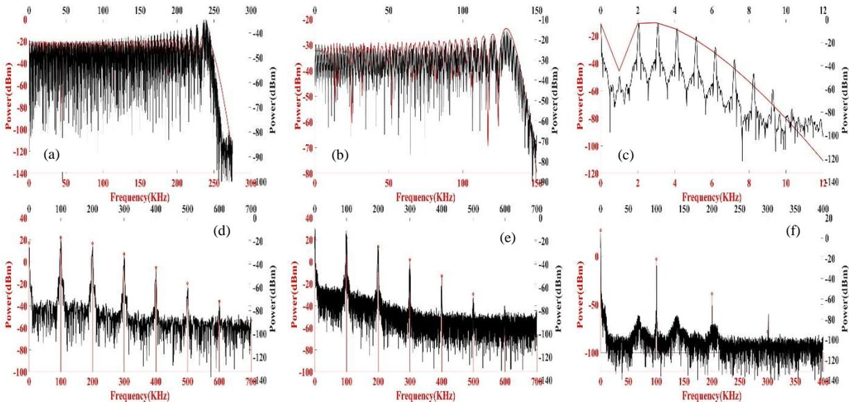
Fig. 2. Comparison of theoretical simulations (red trace) and experimental data (black trace) of output of electronic frequency divider for different division ratio and for different modulation format at input. (a) divide by 1 of FM, (b) divide by 2 of FM, (c) divide by 64 of FM (d) divide by 1 of PM, (e) divide by 2 of PM, (f) divide by 32 of PM.
