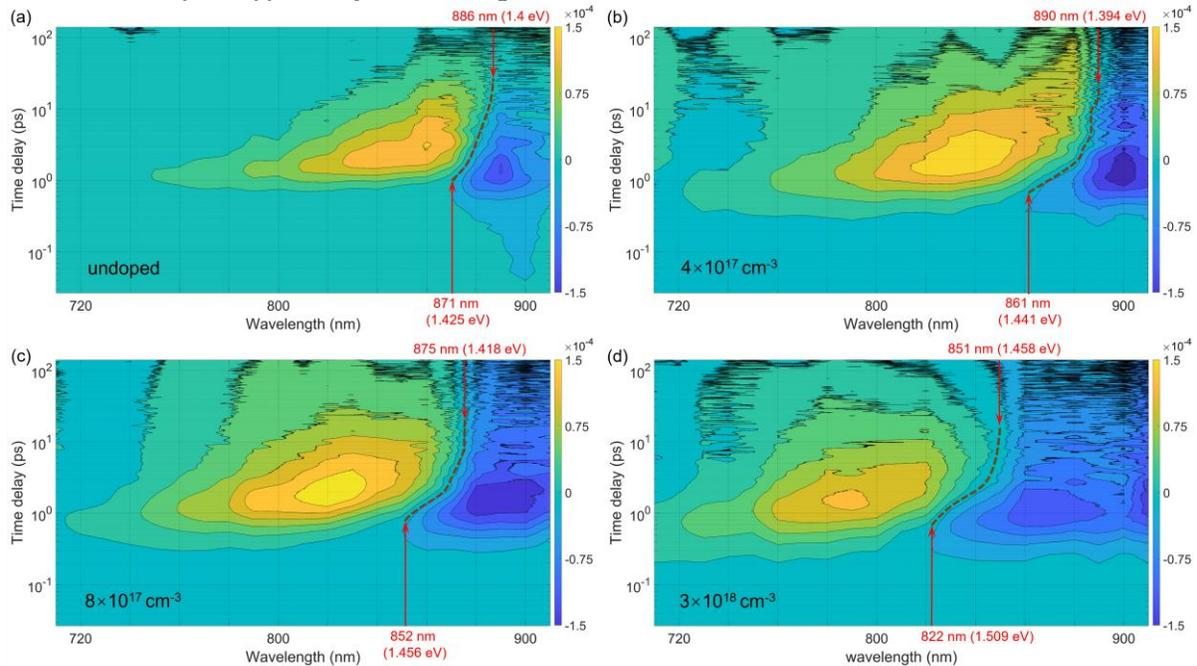
**Fig. 1.** 2D contour maps of the transient dispersion in GaAs wafers, measured by our few-cycle PPR system. Four samples with different doping concentrations are used: (a) undoped; (b)  $4 \times 10^{17} \text{ cm}^{-3}$ ; (c)  $8 \times 10^{17} \text{ cm}^{-3}$ ; (d)  $3 \times 10^{18} \text{ cm}^{-3}$ . Blue-shifted and steady-state band gaps are labeled.
