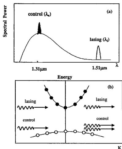
**CThR4 Fig. 2.** Principles of the gain-transparent modulation. (a) optical spectrum, (b) E-K diagram.
