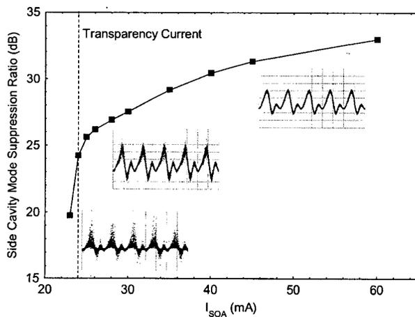
CThR5 Fig. 2. Side cavity mode suppression ratio increases with the driving current of the SOA.
