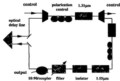
**CThR4 Fig. 1.** The experimental set-up of the mode-locked ring laser.
