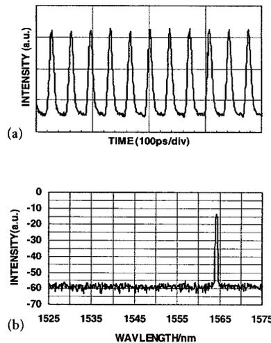
**CThR4 Fig. 3.** Mode-locked output pulses with a repetition rate of 5.7 GHz. (a) pulse waveform, (b) spectrum.
