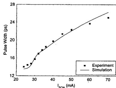
CThR5 Fig. 3. The uncompressed output pulse width varies with the driving current of the SOA.
