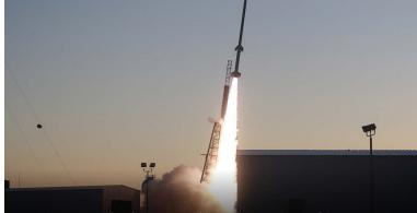
Terrier-Improved Malemute sounding rocket carrying RockSat-X student-developed experiments launched from the launch rail on Wallops Island.
