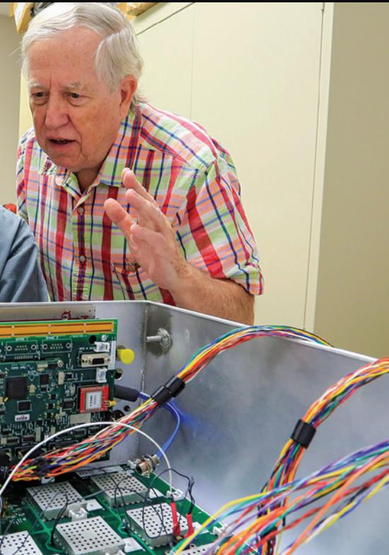
▲ Mike Stewart, left, and Hugh Christian work at the NSSTC on wiring the Fly's Eye GLM Simulator (FEGS) shortly before shipment. FEGS has 30 photometers set to specific wavelengths of light and a wide-spectrum camera. It's flown on an aircraft above the cloud tops and was first used to validate GLM's performance.
