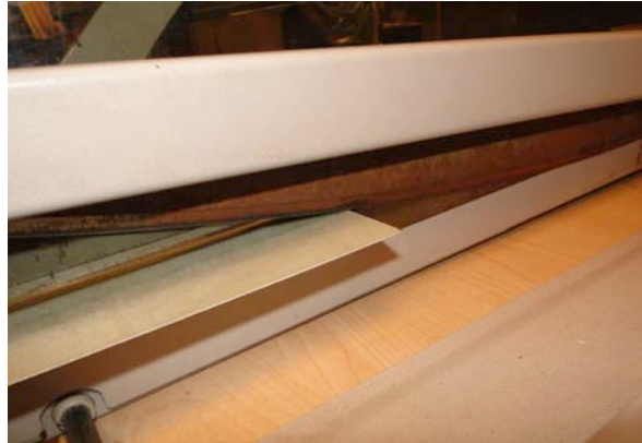
Figure 20: Shearing the Fiberglass Photo provided by J. Dingler.
