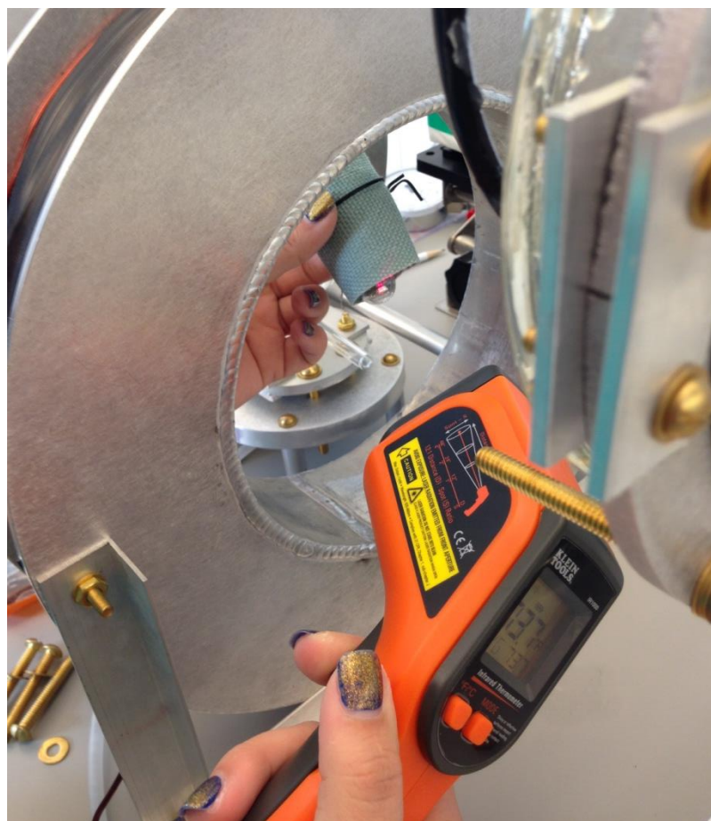
Figure 5. Temperature Measurement of Glass Ampoule
