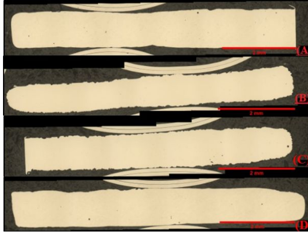
Figure 4. Roughness comparison for the following samples: (A) CAVF, (B) CAVF/CM, (C) CM, (D) CM/CAVF
