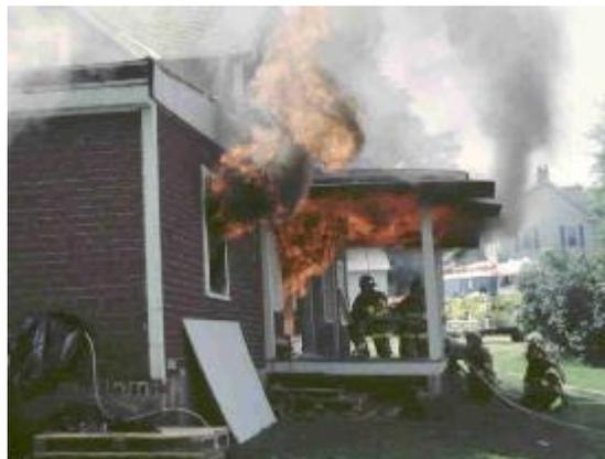
beyond flashover and conditions in other parts of the building will deteriorate rapidly as large quantities of heat, smoke and carbon monoxide are pumped from the fire room after flashover. Without intervention, the time from ignition to flashover can be as brief as a few minutes in many realistic fire scenarios.
