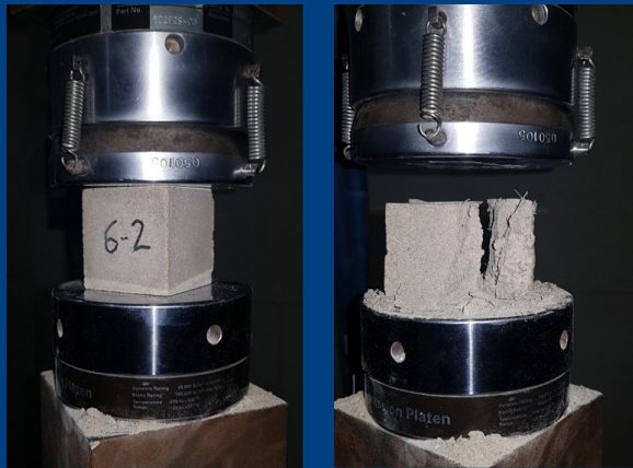
Compressive strength test of potential lunar concrete material that can be manufactured using in-situ materials
