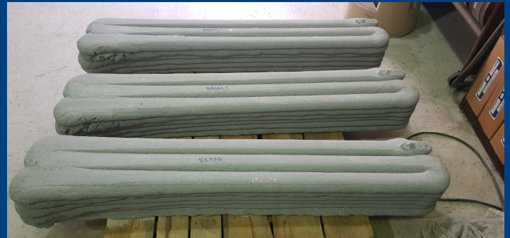
3D-printed concrete beams
