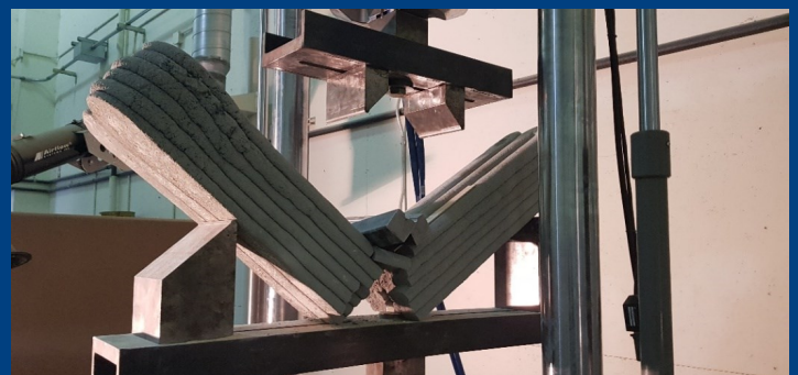
Failure of 3D-printed beams
