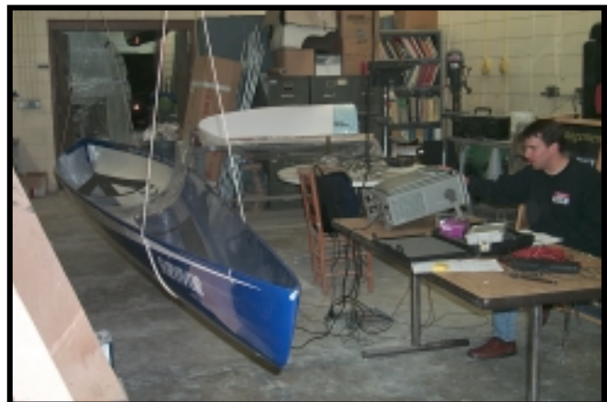
Figure 2. “SURVIVOR” being modal tested.
