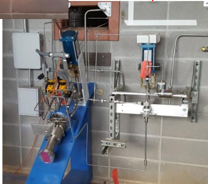
LOX – RP Engine on Test Stand
