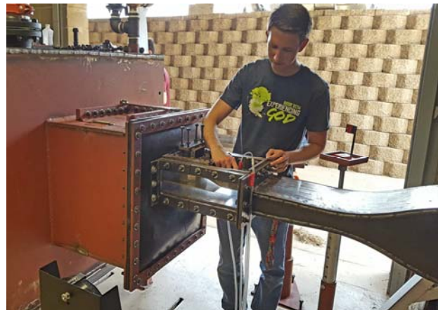
Figure 9. UAH Supersonic Wind Tunnel Test Section
