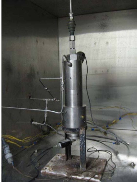
Figure 2. Picture of combustion bomb inside the environmental test chamber.
