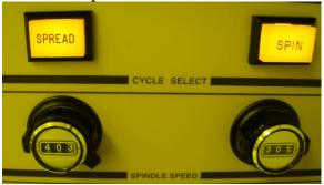
Set the spread and spin speeds using their respective dial adjustments. They are multiplied by a factor of 10 so a spin speed of 300 indicated will be about 3000RPM. Set the desired spread and spin times using the timers below each dial. The maximum spread cycle time is 99.9 seconds and the maximum spin time is 999 seconds. Place the cover on top of the spinner in the event the sample comes off. With all of the spin parameters set press START
