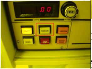
To check how well the sample is centered set the spread speed to about 500 RPM by adjusting the dial below the illuminated SPREAD button so that it displays about 50. If the SPREAD button is not lit press it once which enable a spread cycle and set the timer for about 20 seconds, just enough time to see observe the sample as it spins.
