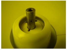
Put your sample on the chuck and try to center it. A well centered sample will be less likely to come off during the spin and will result in a more uniform coating. Press the VACUUM button to pull vacuum on the back of the sample. The orange vacuum interlock light should turn off.
