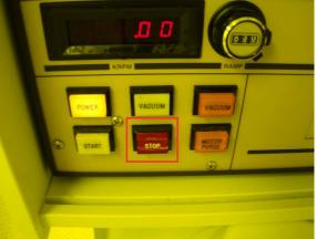
Press VACUUM to release vacuum, adjust your sample as necessary, press VACUUM again to reactivate it and try it again.
