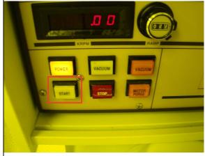
When the spin is complete remove the cover, press VACUUM, remove your sample, clean out the bowl, recover the spinner and press POWER to turn the machine off.
