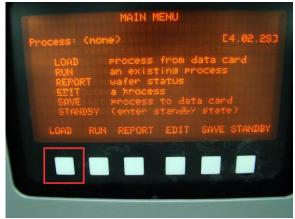
Use the proper magnetic card for the process you wish to run and follow the on-screen directions
