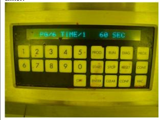
Multiple spin stages can be programmed by repeating the above steps for each stage.
