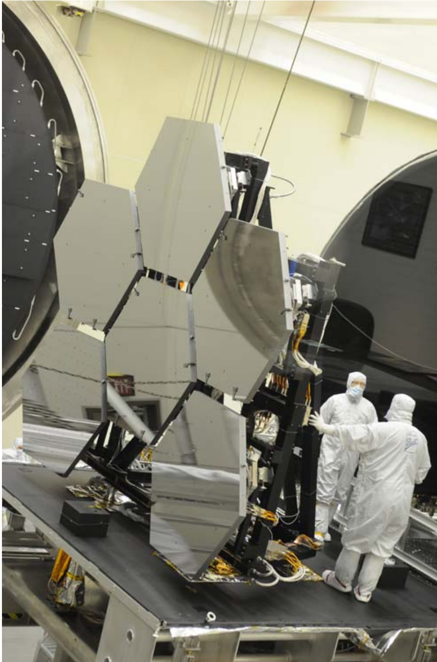
Scientists inspect telescope mirrors at NASA-Marshall Space Flight Center's X-ray and Cryogenic Facility.
