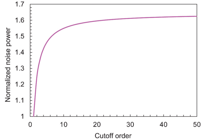
FIG. 2. (Color online) The dependence of the normalized noise power, which is defined as the total noise power over the power of the first normal mode on the cutoff order. \phi_0 = 0.01 is assumed in the computation.
