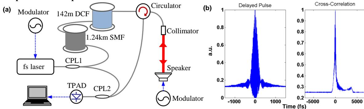
**Fig. 1.** (a) Schematic of the OSCAT lidar. CPL, optical coupler; DCF, dispersion compensating fiber; SMF, single-mode fiber; and TPAD, two-photon absorption detector. (b) Autocorrelation of the delayed pulse and the cross-correlation of the delayed pulse and reference pulse.
