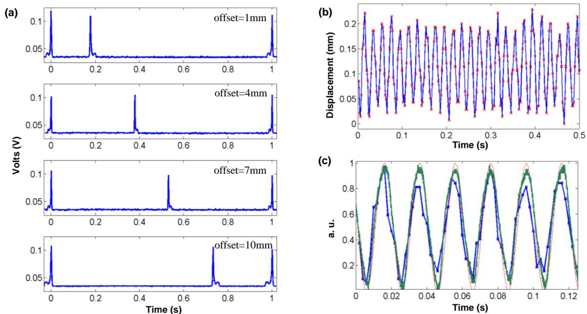
**Fig. 2.** (a) Cross-correlation traces with various target displacements from the reference point; (b) OSCAT-measured displacements (check markers) when the target oscillates at about 50 Hz along the line-of-sight direction; (c) Comparison between the OSCAT-measured target trajectory (blue) and the trajectory given by the optical power method (green) as well as the modulation signal (red) applied on the speaker.
