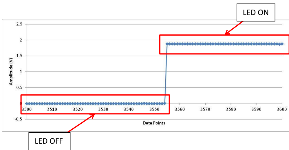
Figure 10: Baseline Voltage Data
