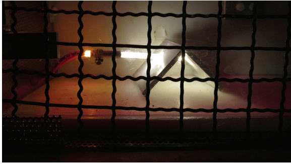
Figure 6. Stainless steel shield and pin ignition at 440 W.
