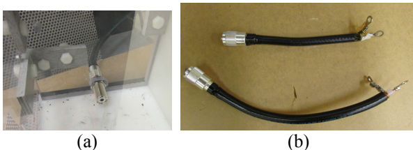
Figure 11. (a) Polycarbonate containment with and female-female connection. (b) Dipole connectors for inside the polycarbonate containment to connect female-female connector to antenna design.
