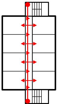
Delivery of water to each corridor is via "riser" pipes. These risers are typically installed, along with drainage pipes and system test assemblies, in exit stairways, where aesthetics are not as important. In many buildings, standpipes are already located in the stairways and can be converted to combined sprinkler-standpipe risers.
