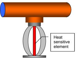
Contrary to popular portrayals in the media, sprinkler systems do not activate when somebody pulls the fire alarm or when a smoke detector activates. Nor do all sprinklers open simultaneously when the first one activates. Each sprinkler has its own heat sensitive element that must be heated to its activation temperature of about 165°F before the sprinkler will operate. This heat sensitive element holds a cap in place over the sprinkler's orifice.
