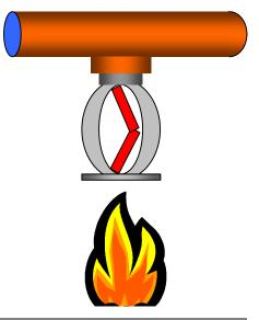
Once activated, a sprinkler discharges water at a rate of approximately 20 gallons per minute in a fairly uniform spray pattern throughout the room. This water spray cools the fire environment while wetting fuels surrounding the fire source to prevent or retard their ignition. In this way, the fire is held in check until the fire department can respond and complete extinguishment of the fire.
