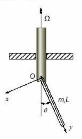
Find the free response of the following two-degree-of freedom system using modal analysis method. Give answers in terms of natural frequencies, the corresponding mode shapes (give schematics), and the time response of the coordinates.
