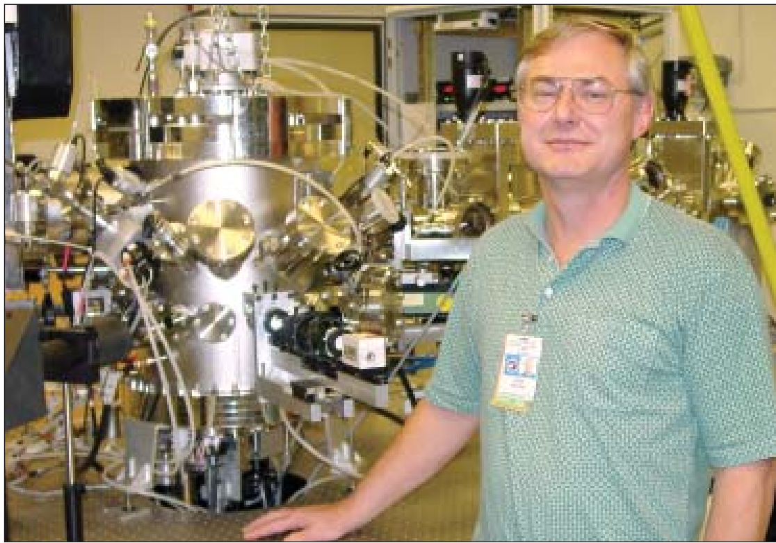
Tom Rathz, above, and the new electrostatic levitator at NASA's Marshall Space Flight Center. The tiny samples being levitated — the pellets in the vial, left, are sapphires — are heated by laser until a molten bead is floating in mid-air.
