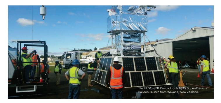
In late April, NASA's Extreme Universe Space Observatory Super Pressure Balloon (EUSO-SPB) took flight from Wakana, New Zealand, carrying a new telescope designed to detect ultra-high-energy cosmic rays interacting with the Earth's atmosphere.
